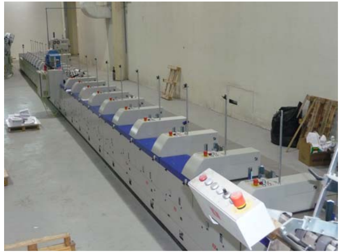
The Kolbus model ZU 841 gathering machine with 24 stations coupled with the KM421C.
