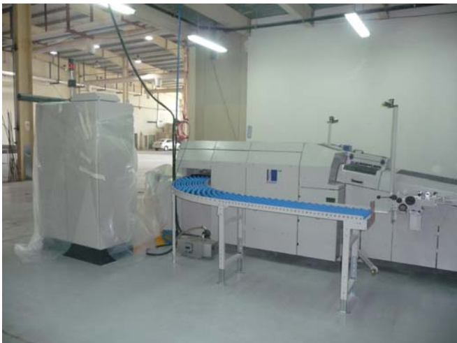
The Kolbus casemaker DA 260 for the making of the hardcover for books.
