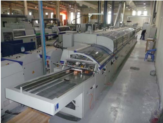
The Kolbus perfect binding line includes the KM 412C binder with the conveyor and cooling/drying system as well as an inline three Knife Trimmer HD 153P.
