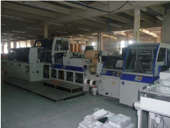
A BF 512 has equally been ordered for the rounding, backing and casing-in of book blocks in hard, flexible and plastic covers and subsequently pressing and joint-forming of books.
