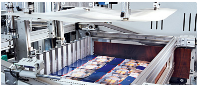
Once a complete layer of delivered stacks has been formed onto the pallet, paper/cardboard sheets are automatically placed on the layer to stabilize the pallet stack.
