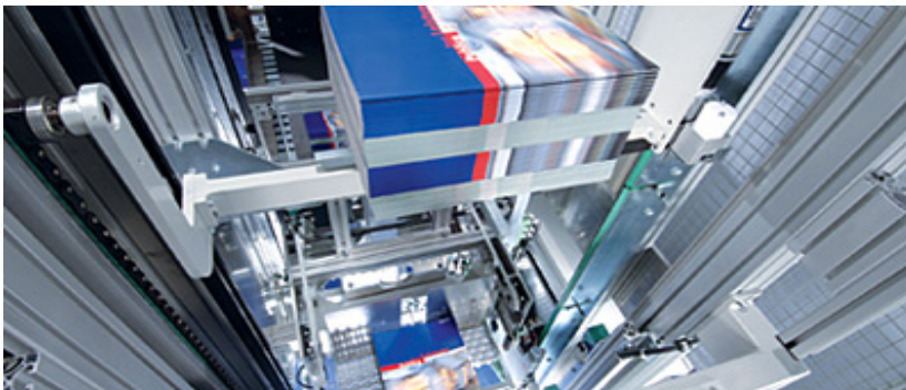
The Paternoster system saves space and transports the products to a specified palletizing height
