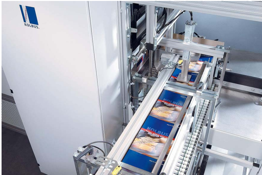
The XBV KOLBUS bundle wrapping machine can be universally used for shrink wrap packaging or as a stretch packaging unit for simple, economical protection during transport.
