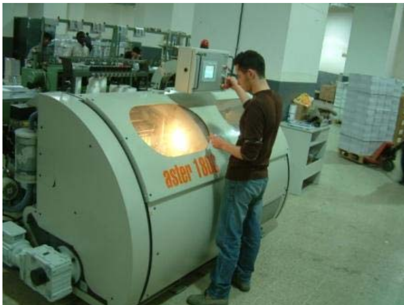
The Aster 180 C at the Typopress premises in Jdeideh – Lebanon. Two large oval windows make it easy to overview the machine operation.
