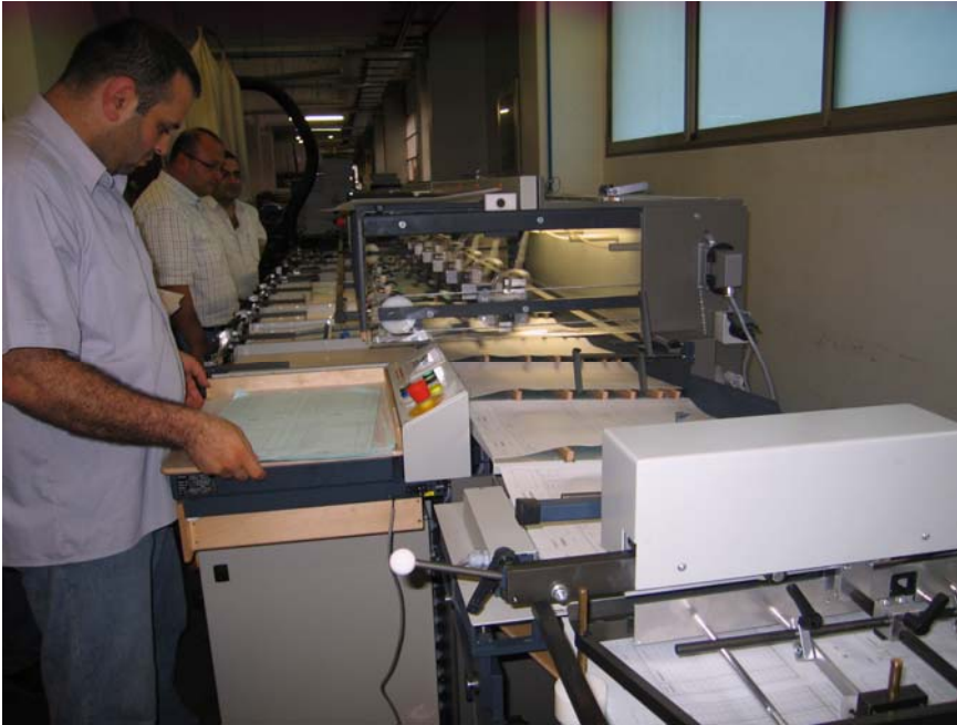
The tb sprint is equipped of up to 16 individually adjustable suckers at each station for an optimal suction
