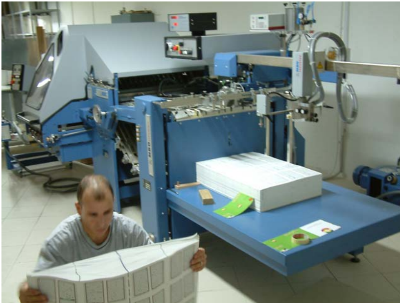
One of the MBO combi folding machine's major assets is that the height of the knife can be adjusted and aligned without any tools and during the production process.
