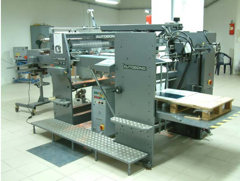
Al Arz's Mini 76 TH thermal laminating machine is fitted with a rising pile back separation stream feeder, a sheeter and a jogging table.
