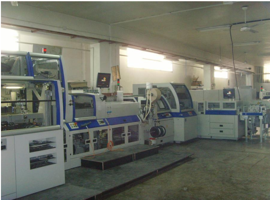
The fully automatic compact Kolbus Book Production Line BF 512, with integrated forming and pressing machine.
