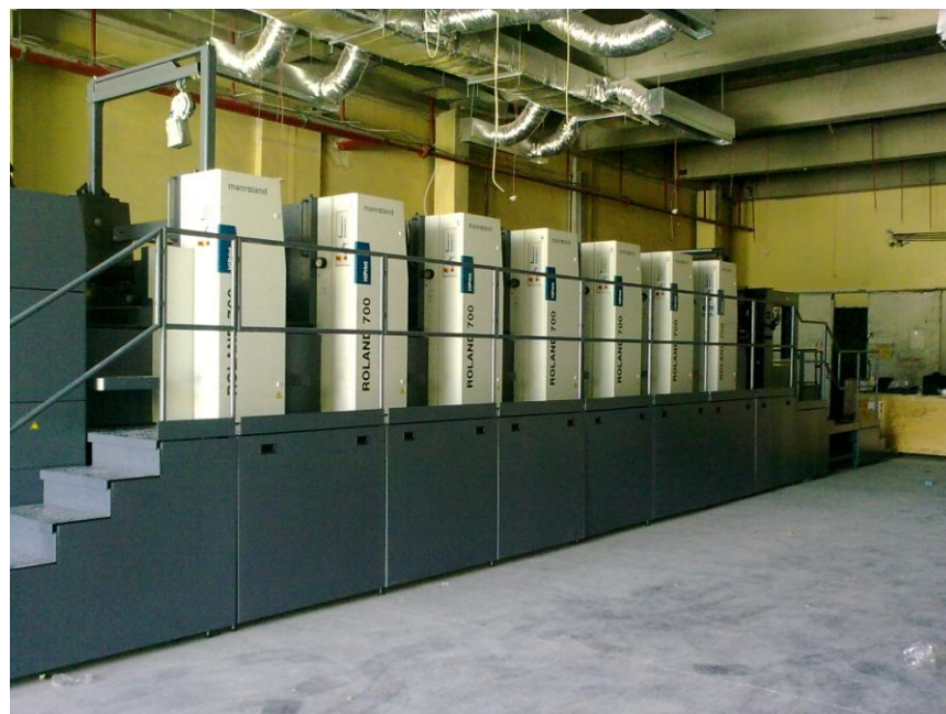
The ROLAND 706 LV at Perfect Printing Press in Jordan installed by Dynaserv Service Engineers
