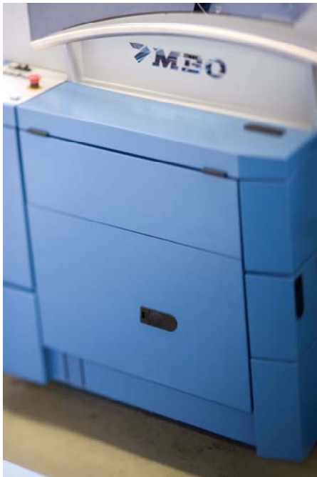
Fully encapsulated design: The opening for infeed and outputs were reduced to the absolute minimum in terms of size
