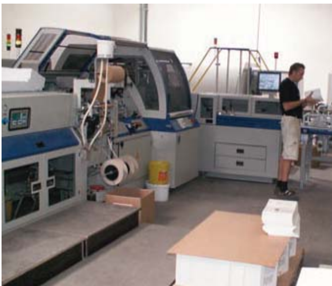
Machine operator Christoph Grybsz knows no other speed on his book production line BF 511 at Connexus than 30 cycles/min.
