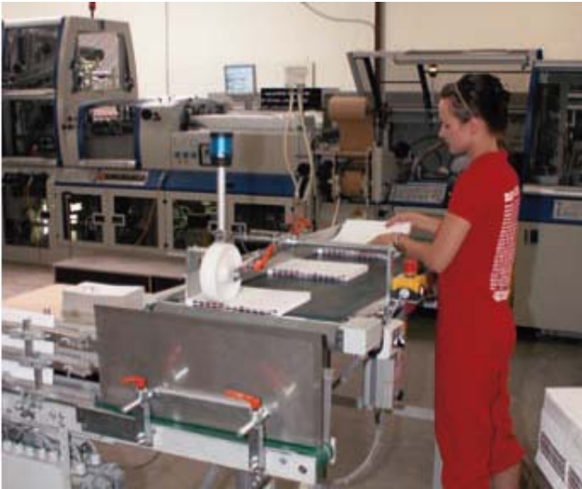
An employee at Connexus GmbH positions book blocks in the Sigloch gluing line, which boasts a long drying zone.
