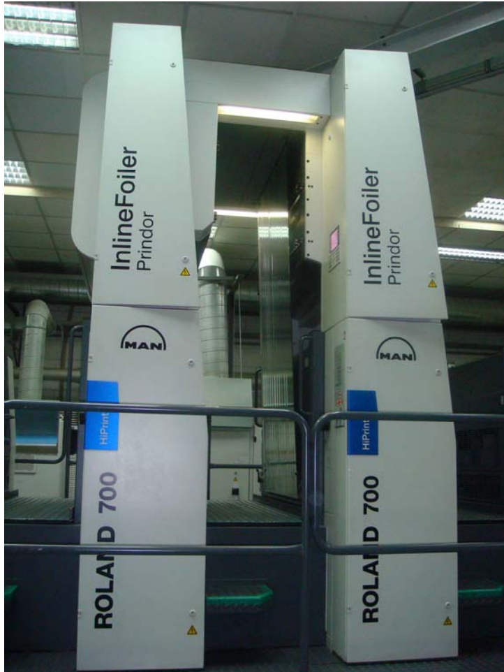
Above pictures show the InlineFoiler Prindor at British Industries installed on the R706 LTTLV.
